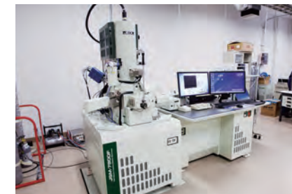
Scanning Electron Microscope System and Cross Section Polisher
