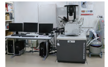
Focused Ion Beam/Scanning Electron Microscope Dual-beam System
