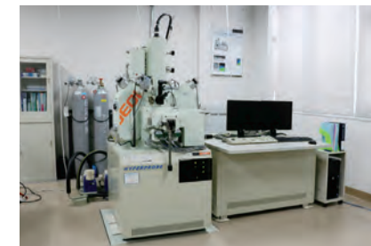
Field Emission Electron Probe Microanalyzer with SXES
